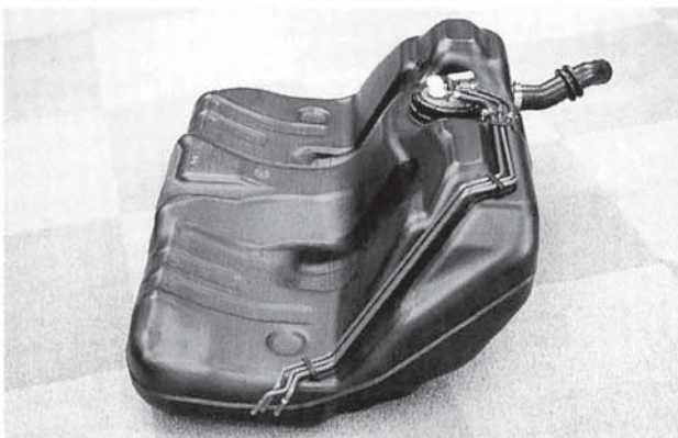
Photo14.1-18 Fuel tank (HDPE/Adh./PA/Adh./HDPE)
