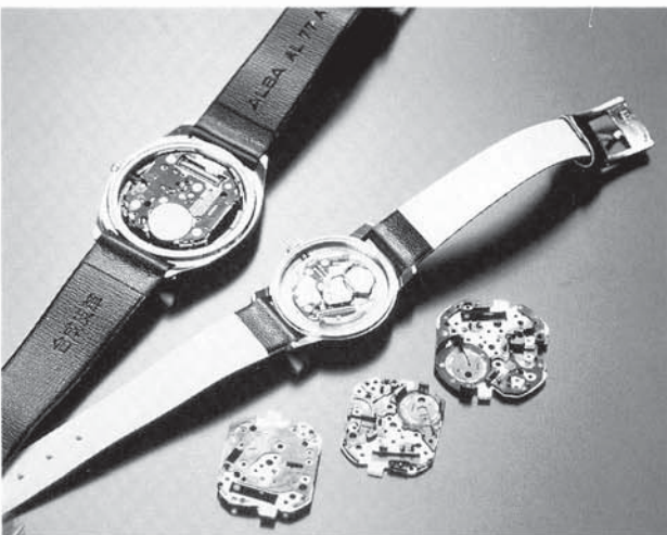
Photo14.3-4 Wrist-watch mechanical parts and gear (POM)
