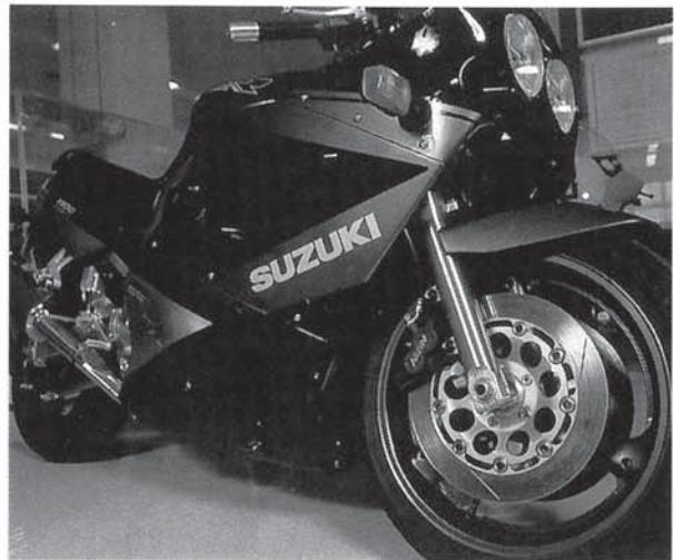
Photo14.1-51 Motorcycle cowling (GF-PA)
