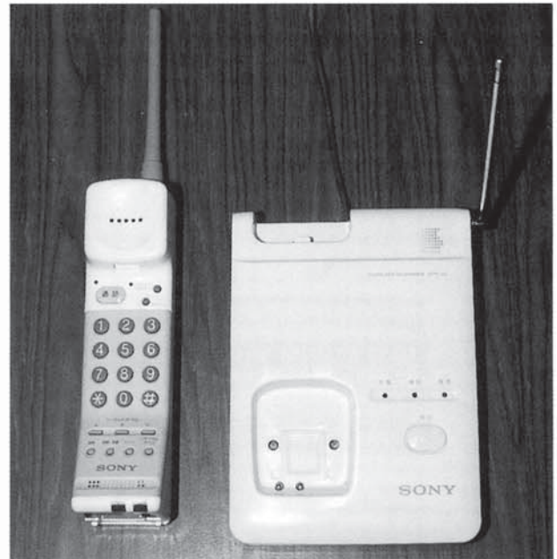
Photo14.2-68 Cordless handset/antenna sheath (TPEE)
