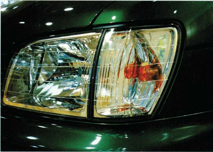
Amber cap of turn signal lamp (PAR)
